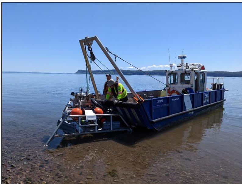
Figure 8: The cabled subsea platform developed for the VITALITY project just prior to deployment at the FORCE test site.
